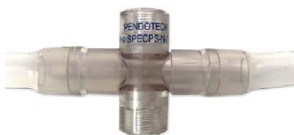
Flow Cell with tubing installed
