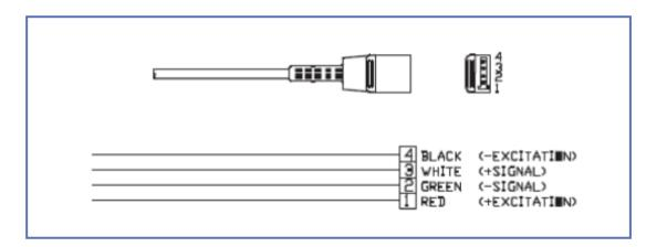
Reusable Cable which connects to the monitor/control system has five wires- four as shown above and the 5th which is a cable shield (silver)
