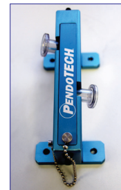
6.5cm single use flow cell installed in stand
