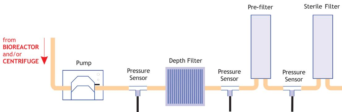
Fig. 1 Single Normal Flow Filtration Train
