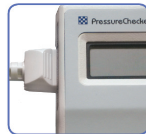
Sensor simulator port for testing monitors only
